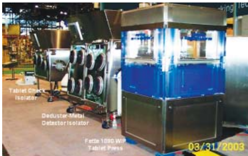
Contained potent tableting process (from Carlisle Life Sciences; photo shows Fette model 1090 WIP tablet press).
