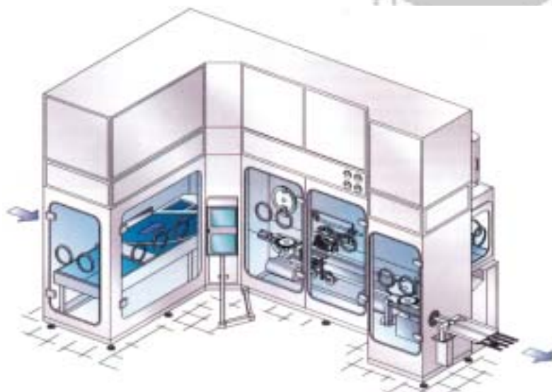
Photo and sketch of FLM 4080 liquid filler with barrier isolator (introduced in 2002 by Bosch Packaging Technology).
