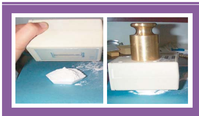
Figure 1: The TC Probe sensor is inverted on top of a container of powder sample.
