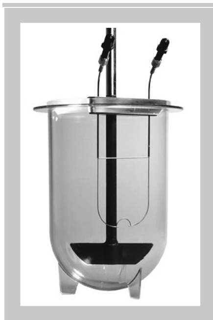
Figure 1: The Arch fiber-optic transmission probe.
