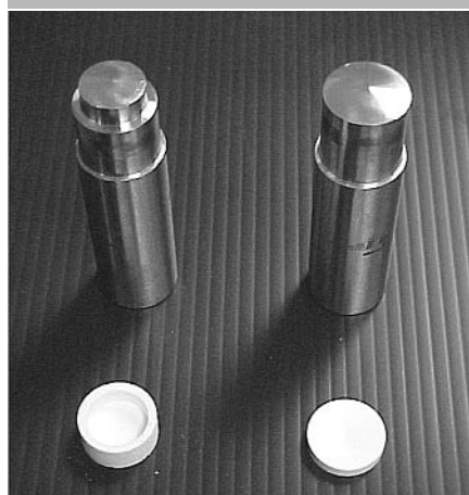
Figure 2: Photo of the tooling used to demonstrate proof-of-concept, a cup, and a finished dosage form.
